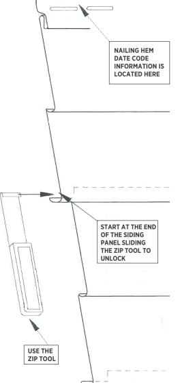
A Date Code is located on the Nailing Hem of all Georgia-Pacific Vinyl Siding panels. This Date Code provides information that will identify date and time of manufacture, as well as, the specific plant of manufacturer. This information is required to process your claim.
